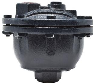
There is no question in our opinion: these are the most reliable air eliminators money can buy. Stainless steel float and mechanism, Viton A seal, 3/4" NPT in and out. (1/2" on special order), 1/16" air outlet orifice operates up to 208 psi. Air release rate at 150 psi is 6.04 cfm. Larger orifice sizes: 3 available on special order but operating pressures decrease. Structural pressure rating is 250 psi on all models. Repairable replacement parts are available.
