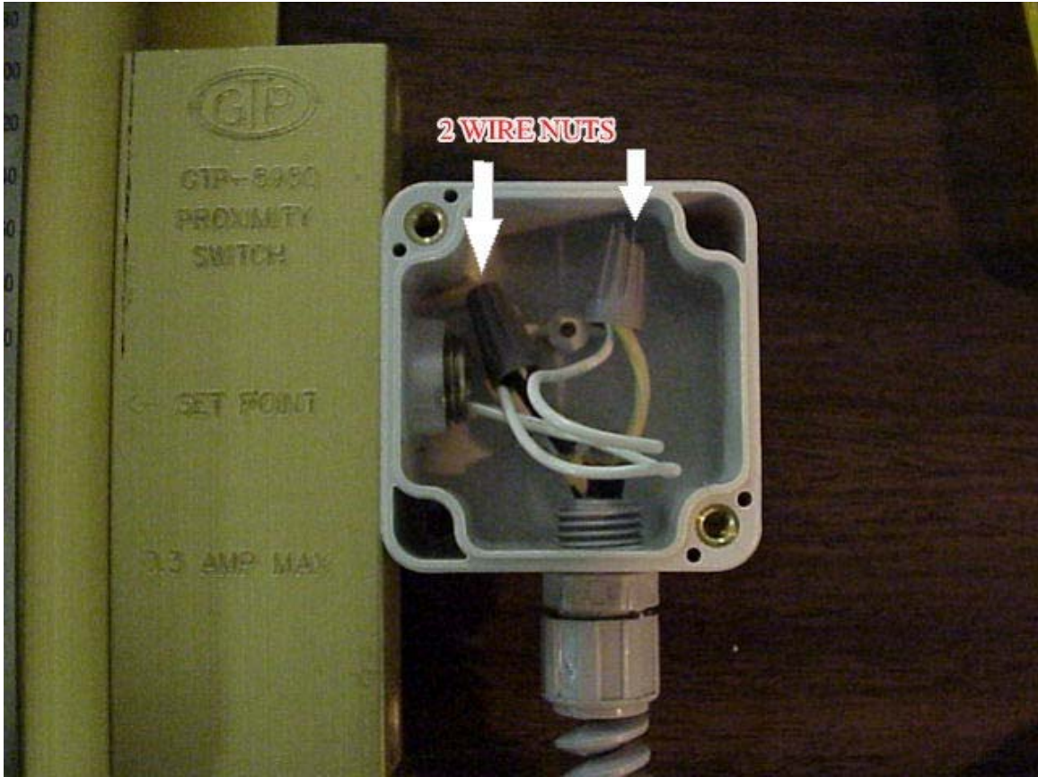
Remove one of the two wire nuts. It does not matter which one.
