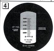
Read the measurement value where the boundary line intersects the scale.
